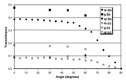
Fig. 2: Angle dependent energy transmittance of a triple glazed gasochromic IGU (t<sub>e</sub> solar transmittance; g total solar energy transmittance; q<sub>i</sub> secondary heat gain factor; (b) bleached state; (c) coloured state (Source: Fraunhofer ISE report to SWIFT, cited in [10]).
