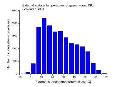
Fig. 4: Distribution of the external glazing surface temperatures for gasochromic triple glazed units in the coloured state, tilted 45° and orientated south for outdoor exposure tests at Freiburg, Germany. 5-minute averages, December 2001 to June 2002. (Source of data: Fraunhofer ISE).
