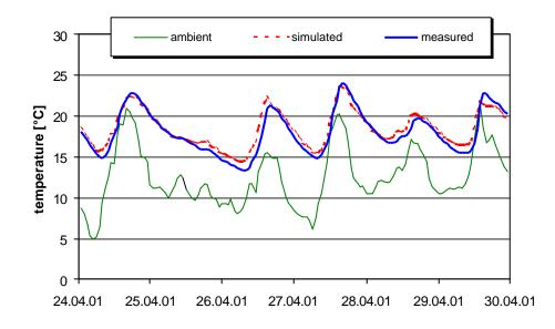
Fig. 3: Comparison of measured and simulated air temperatures in the FASTEST test cabin equipped with gasochromic glazing (Source: Fraunhofer ISE report to SWIFT).
