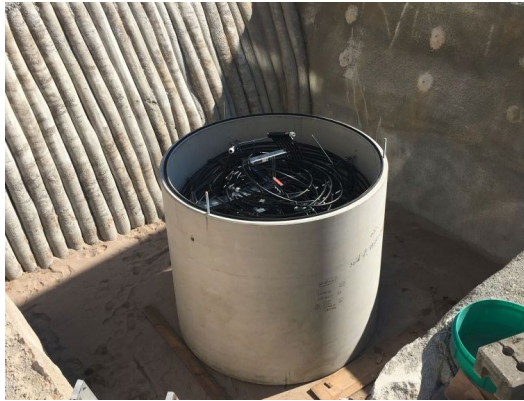
Experimental ice store at the Institute for Building Energetics, Thermotechnology and Energy Storage (IGTE) at the University of Stuttgart (Germany) with a water volume of 10 m 3 and heat exchangers e.g. for testing sensors to determine the state of charge (Source: IGTE)
