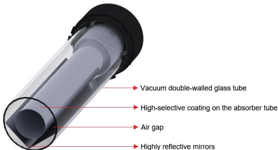
Figure 1: Cross-Sectional View of a double-ends open Evacuated-Tube (Source: airwasol GmbH & Co. KG).
