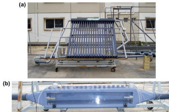
(a) The evacuated-tube air collector: overall view of the experimental set-up; (b) the drying chamber (Chr. Lamnatou et al. 2012).
