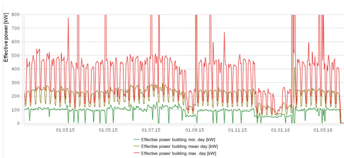
Figure 9: Base, mean and peak load building efficiency
