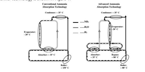
Figure 1: Advanced (Low Temperature) Ammonia Absorption Chiller versus conventional ammonia diffusion absorption chiller – Schematic
