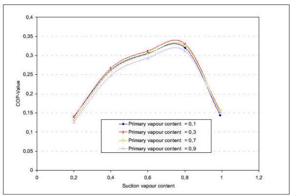
Figure 3: COP versus vapour content of the secondary flow, on suction side of the ejector, at various vapour contents of the primary flow for a composition of 99% ammonia and a mixing section efficiency of  $?_{M} = 0.7$  (the mixing section is part of the ejector).
