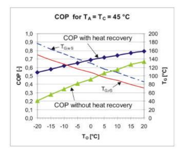
**Figure 2:** Coefficient of performances (COP) of the DACM with/without heat recovery for evaporator temperatures from -20 up to  $+20^{\circ}$ C and for  $T_A = T_C = 45^{\circ}$ C (simulations).
