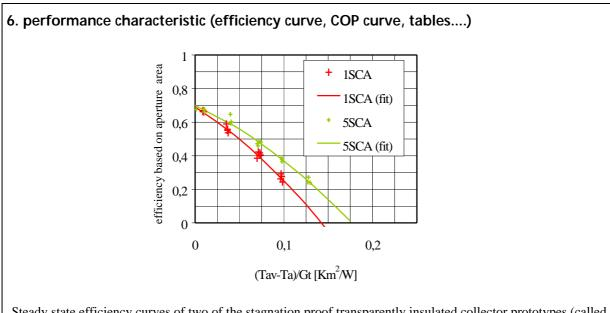
Steady state efficiency curves of two of the stagnation proof transparently insulated collector prototypes (called 1SCA and 5SCA, for use up to 90°C and 120°C respectively).
