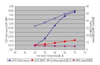
Figure 2: COP<sub>heat source</sub>, COP<sub>booster pump</sub> and cooling capacity versus hot water temperature
