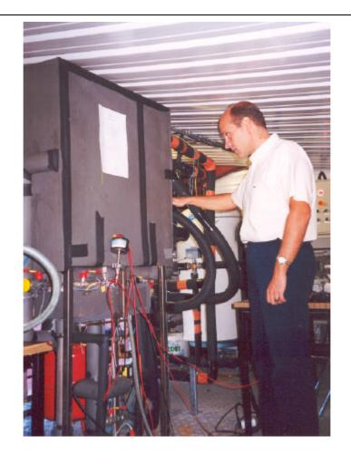
Prototype absorption heat pump
