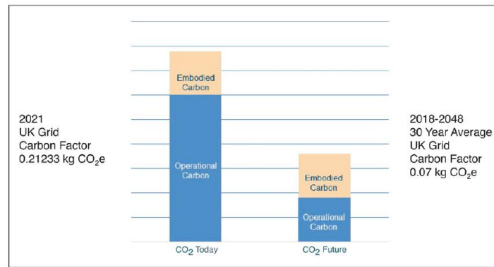
Figure 15: Comparison of embodied and operational CO 2 emissions of a luminaire evaluated using emission factors valid for 2021 ("CO 2 today" and 30-year predictions ("CO 2 Future"))).
