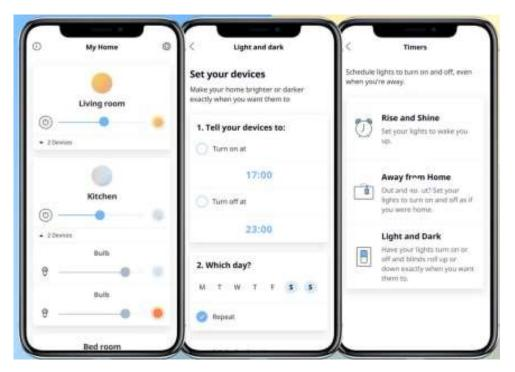
Figure 3. Example of UI: Ikea Smart Home App interface – from left: 1) Dimming of rooms and specific light sources. 2) Setting dynamic control using clock and calendar. 3) Setting dynamic control over lighting by defining scenes.<sup>3</sup>
