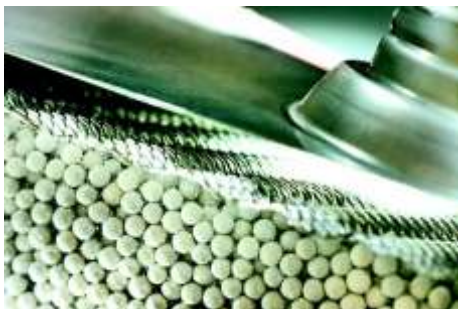
Zeolite beads in the heat exchanger of the zeolite dishwasher. Source: ZAE Bayern
