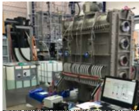
Liquid nitrogen based thermal storage system developed at the Lucerne University of Applied Science. Source: University of Applied Sciences, Lucerne, Switzerland
