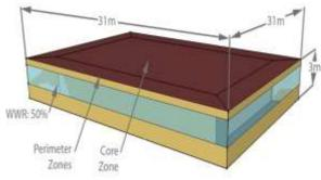
Some assumptions have been made when establishing the insulation values. When there are no requirements for glazing, the R-Value is assumed as a single glazed window. The USA R-values vary between building types due to the nature of the construction: Residential is Timber framed; and Non-residential is Steel – framed construction.
