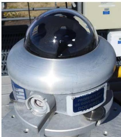
**Figure 3-20. Delta-T Devices, Ltd., SPN1. Image by NREL.**
