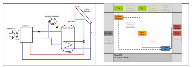
Figure 5: Unified hydraulic scheme (left) and square view (right) of a solar thermal and heat pump system. The system shown applies external air as additional heat source and the two systems are connected in a "serial" and "parallel" way.
