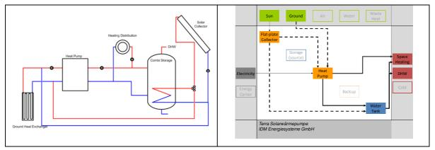
Figure 3: Unified hydraulic scheme (left) and square view (right) of a solar thermal and heat pump system. The system shown applies a geothermal heat exchanger as additional heat source and the two systems are connected in a "serial" and "parallel" way.
