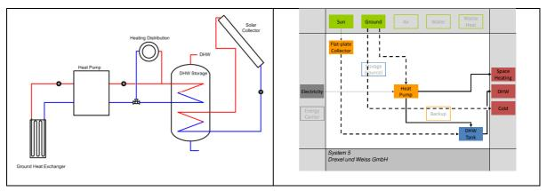
Figure 2: Unified hydraulic scheme (left) and the visualization scheme "square view" (right) of a solar thermal and heat pump system. The system shown applies a geothermal heat exchanger as additional heat source and the solar thermal system and heat pump system are connected in a "parallel" way only.
