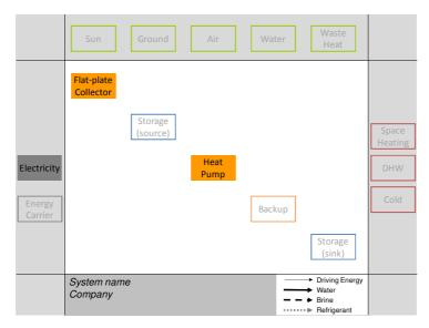
Figure 1: Structure of the "square view" diagram, showing the main components, heat sources, heat sinks and additional energy carriers implemented in a solar thermal and heat pump system.
