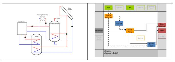
Figure 6: Unified hydraulic scheme (left) and square view (right) of a solar thermal and heat pump system. The system shown applies only the solar thermal collector as heat source. A hybrid collector is used feeding the DHW tank and an ice / water storage.
