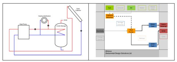
Figure 7: Unified hydraulic scheme (left) and square view (right) of a solar thermal and heat pump system. In the present system an unglazed collector is used serving directly as heat source for the heat pump.
