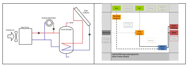
Figure 4: Unified hydraulic scheme (left) and square view (right) of a solar thermal and heat pump system. The system shown applies external air as additional heat source and the two systems are connected in a "parallel" way only.
