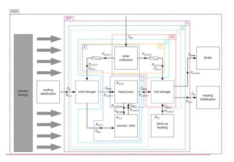
The vision of a system and all possible définitions of performance indicators from S1 to S6, SPF and PER Primary Energy Ratio (Subtask B)
