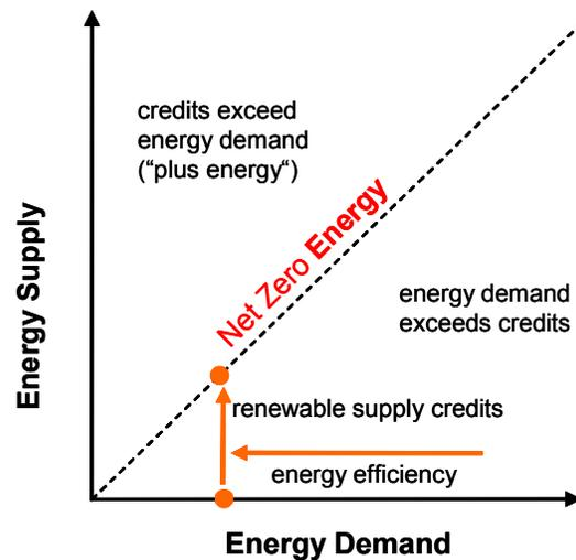
Figure 3. Net Zero Energy is achieved by reducing energy demand to be equal to clean renewable energy supply on an annual basis.
