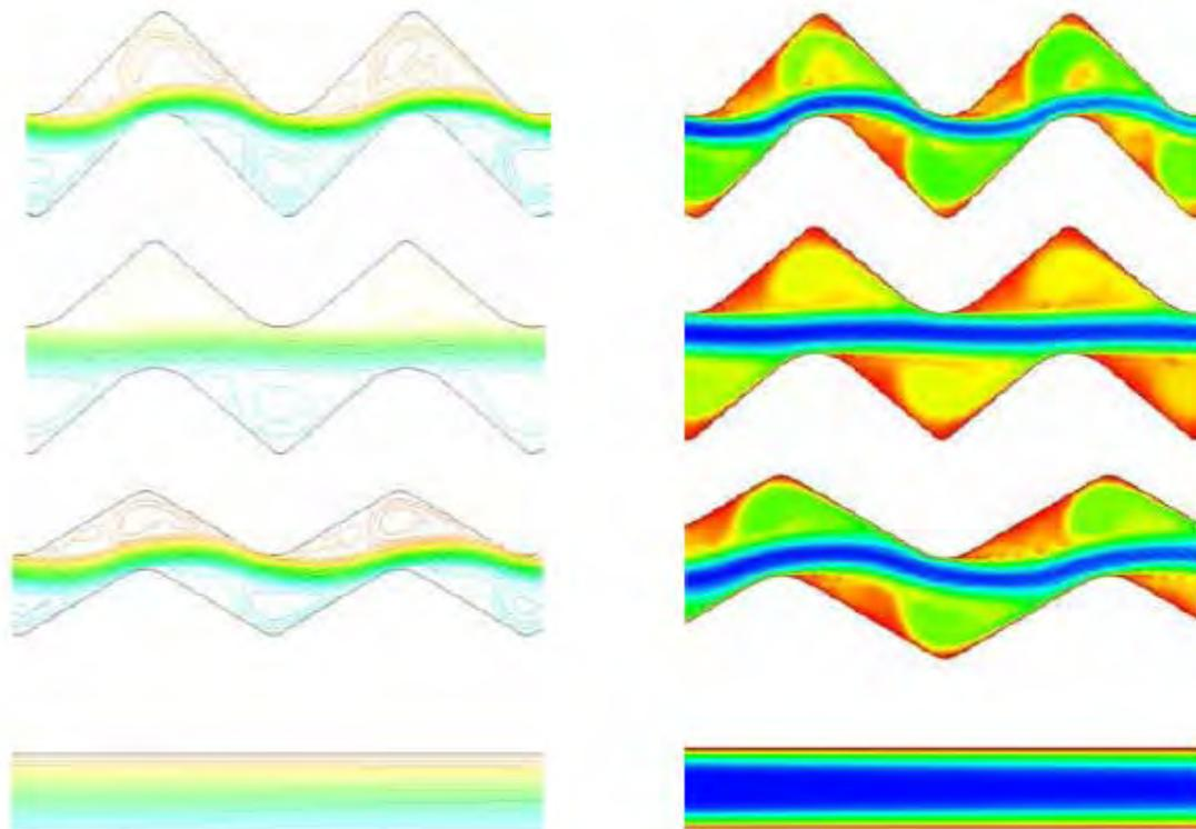
**CFD-simulation of different absorber channel designs Streamlines for liquid heat-transfer-media are shown in the left column, temperature distribution on the right side ( brown color shows hot and blue colors cold regions).**
