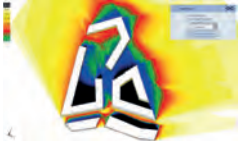
Details on A1 / 1st Variation Problem: Circled building cause extreme shadowing into the inner yard.
