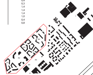
2nd Variation Solution: Remove highlighted building. This allows more sun exposure into the inner yard. Opening for the whole building is located at street and no longer in
