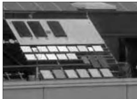
Outdoor-weathering of reflector and absorber samples in Freiburg, Germany.
