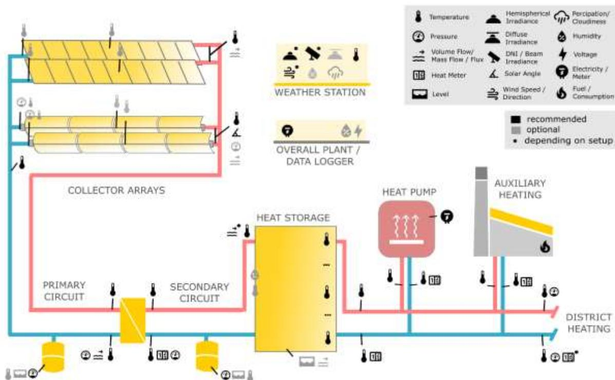
Figure 2: Illustration of a solar district heating plant displaying recommended sensors.
