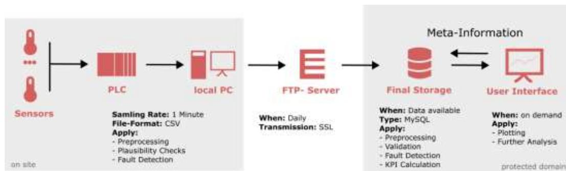
Figure 3: Data flow of example architecture 1.
