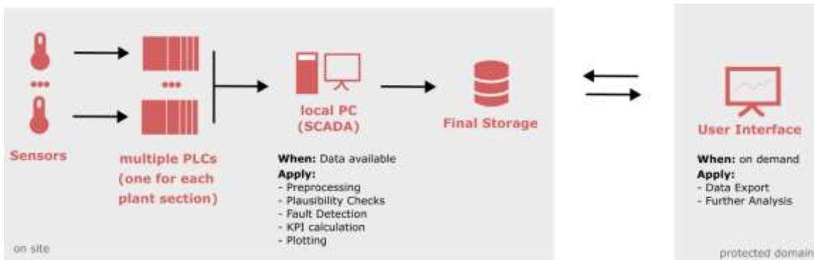
Figure 5: Data flow of example architecture 3.
