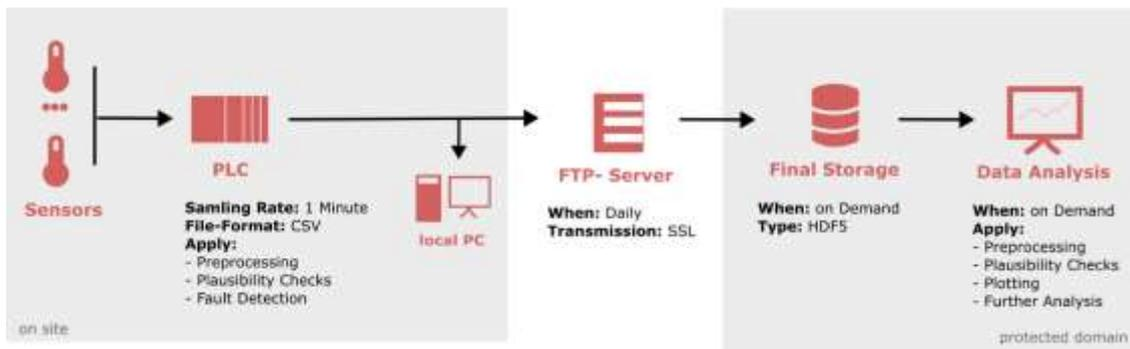
Figure 4: Data flow of example architecture 2.
