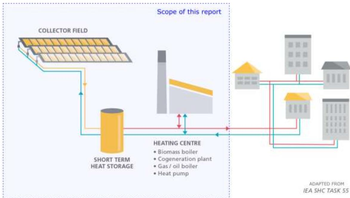
**Figure 1: Illustration of a solar district heating plant with a grey box depicting the scope of this report. Source: adapted from IEA SHC Task 55.**
