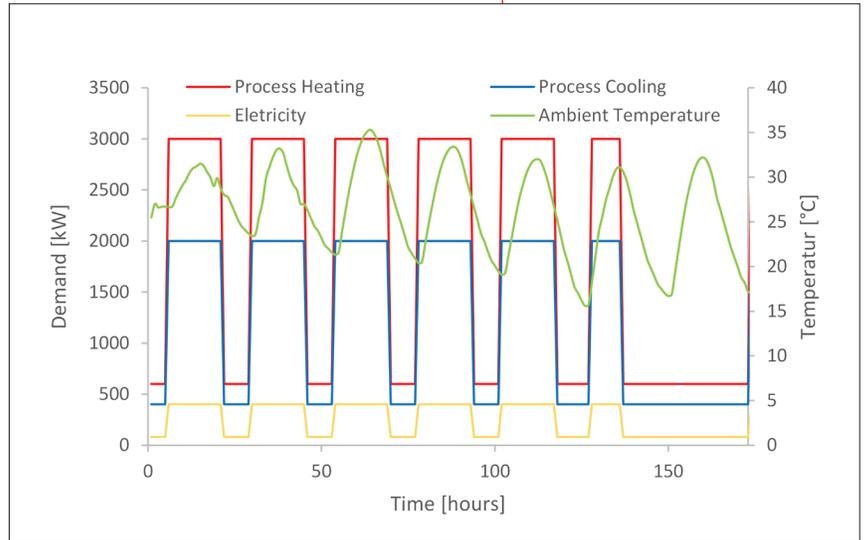
▲ **Figure 1. Plot of energy requirements of the industrial application and the ambient temperature over a week in Windhoek, Namibia.**
